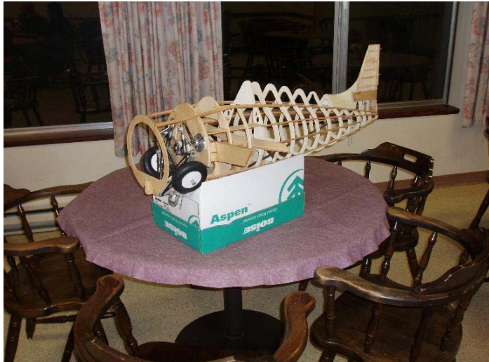
Ralph Suter's Super Secret Patent Pending Scratch built Retracts for his Wildcat.
