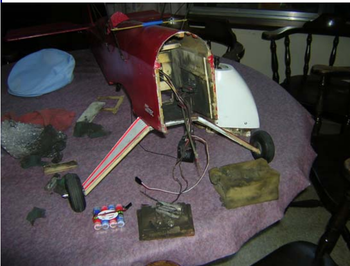
Ted Atmore's Plane after a battery explosion. A good reminder to always be careful when charging your batteries.
